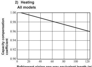
Refrigerant piping one way equivalent length (m)
