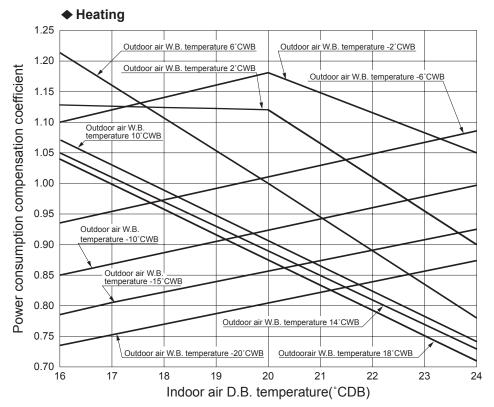
Note (1) The above-mentioned table shows a typical condition among conditions to occur via controlling an air-conditioning equipment.
