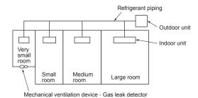
Note(3) The minimum indoor floor area compared with the amount of refrigerant is roughly as follows: (When the ceiling is 2.7m high)
