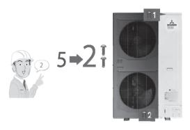
Thanks to improvement of the control box structure by use of hinged board, service and maintenance were made much easier for inverter components.
