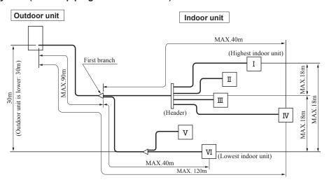
Note (1) A branch piping system cannot be connected after a header system.
