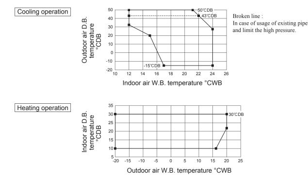
"CAUTION" Cooling operation under low outdoor air temperature conditions
